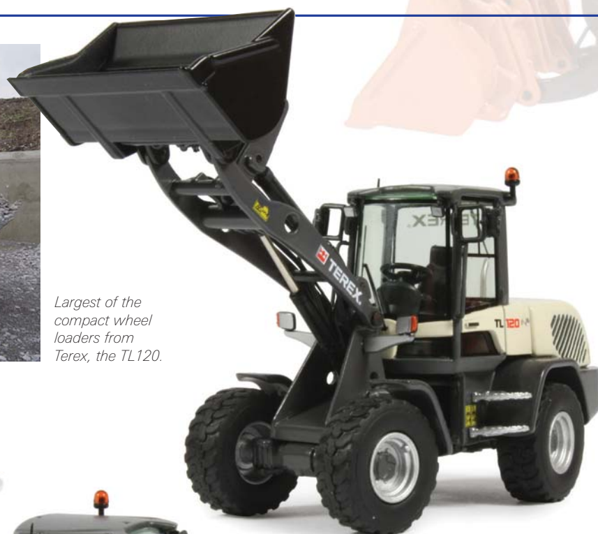
Excellent range of movement of the loader arms and bucket.
