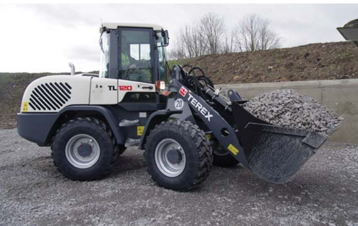
Largest of the compact wheel loaders from Terex, the TL120.
