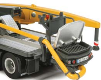
Above: The THP140H pump has an output of 138m 3 /h with a 600 litre hopper capacity.
