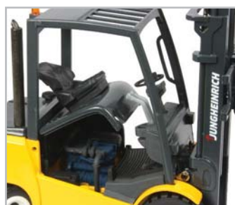
Above: Good cabin detailing with opening side and upper cover revealing the replicated Kubota engine.
