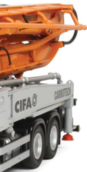
Above: The outriggers are fully functional with lowering jack legs and separate mats.
