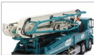
Right: The five section boom folds neatly during transport.
