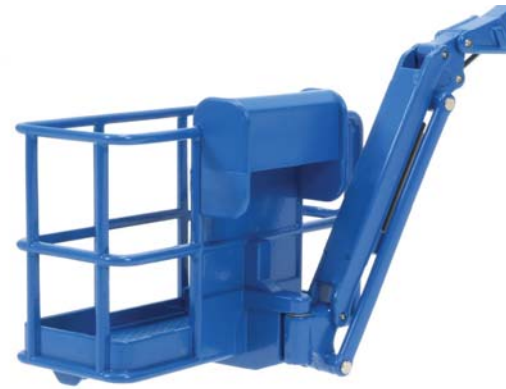
Right: The basket has rotation 900 rotation to each side along with a parallel linkage arm.
