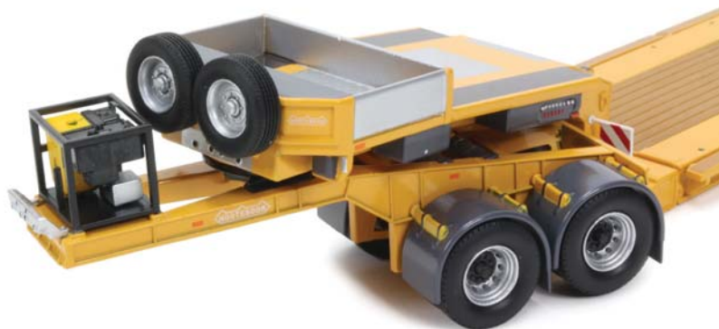
Above: The dolly has a generator and can be disconnected from the gooseneck.
