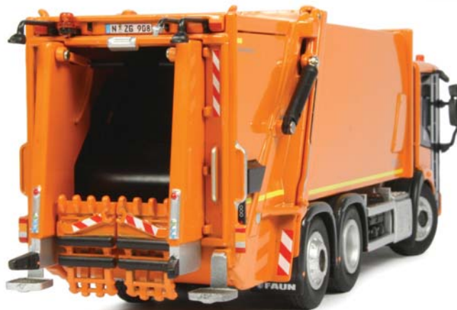
ABOVE: The rear of the model has side platforms and grab handles for the operators.
