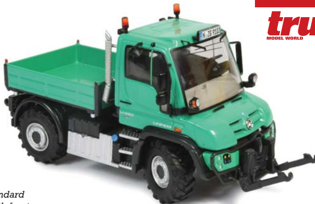
Above & Right: The agricultural version of the U430 has tractor style tyres and both front and rear linkage.
