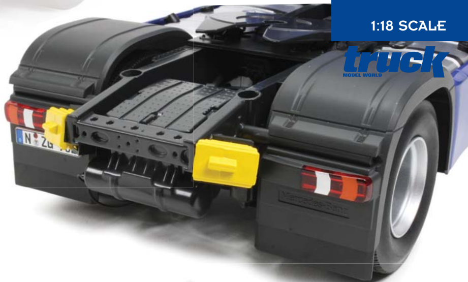
Above: The rear has the air tanks with all the lines added.
