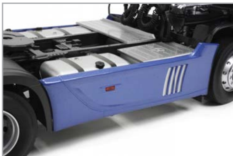
Above: The model has protective side panels covering the small and large fuel tanks and silencer.
