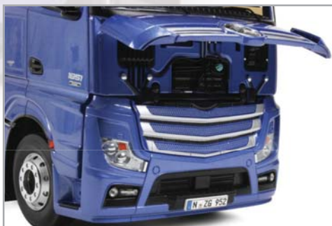
Above: The front grill lifts up to reveal the interior details while the entire cabin tilts forward.
