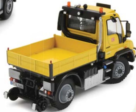
Left: The rail wheels can be raised allowing road operation and the model is fitted with narrow rubber tyres and sloping wheel hubs.
