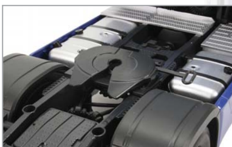
Above: The fifth wheel plate pivots and the lever activates the lock.
