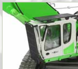
Below: Good surface detailing of the engine panels and rear counterweight plus hydraulically elevating cabin with option to fit platform.
