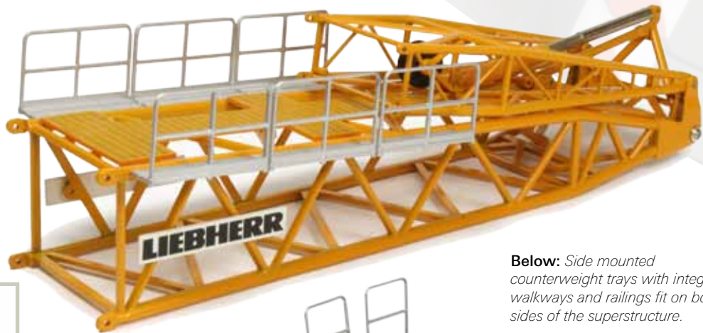
Above: Mesh walkways and safety railings have been added to the working areas of the boom and jib sections..
