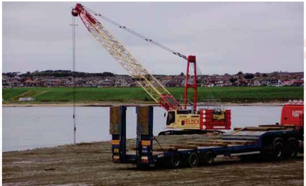
Above: Liebherr HS855HD showing its versatility placing rock armour at Peterhead harbour by Mervyn Walker.
