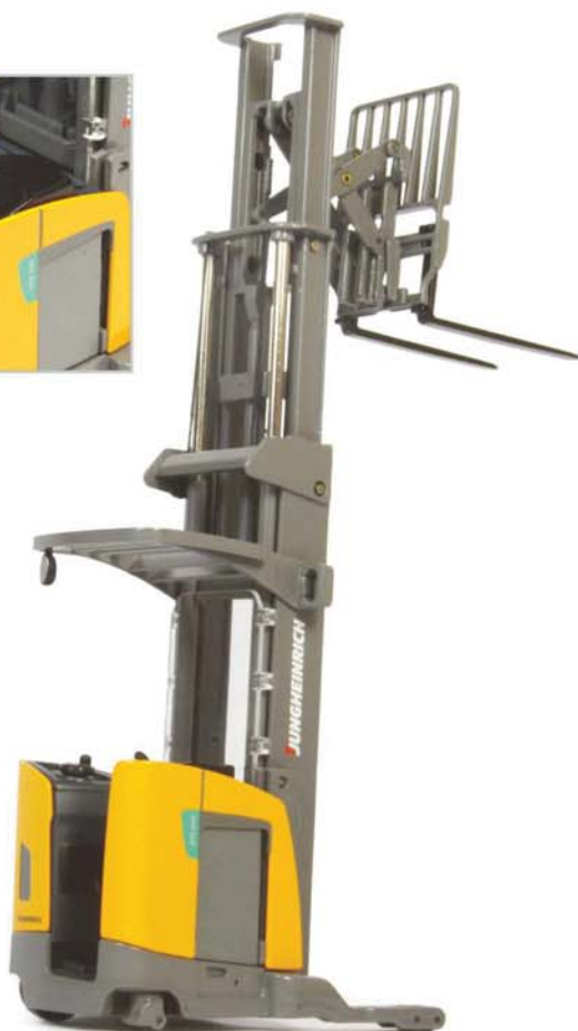
Right: The three-section mast can be raised and lowered, with rope used to operate the stages.
